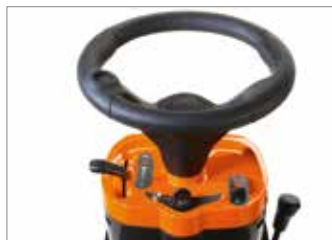
The electromagnetic clutch is engaged quickly and quietly by way of a handy dash-mounted button.
