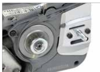
OnBoard clutch: quick fitting of bar and chain, cleaner clutch for lasting performance.
