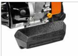
Front ballast that increases the stability of the two-wheeled tractor, particularly on harder terrain.
