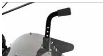
50 cm rotor with depth adjuster.
