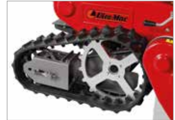
Tracked propulsion system, oscillating on the vertical plane ( 80 TR , 100 TR ).
