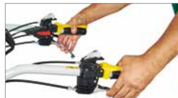
Service and parking brake engages automatically when the clutch is disengaged, preventing accidental dangerous movements.
