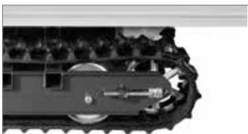
Rugged undercarriage with track tensioner sprocket, perfectly balanced for correct weight distribution and excellent grip on all types of terrain.
