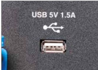
Output with USB socket for charging electronic devices.
