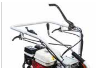
Steering with independently controlled release and brakes.
