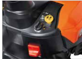
The cutting blades are activated simply by pushing the electromagnetic clutch control button located on the dashboard. This system engages the blade with no kickback.
